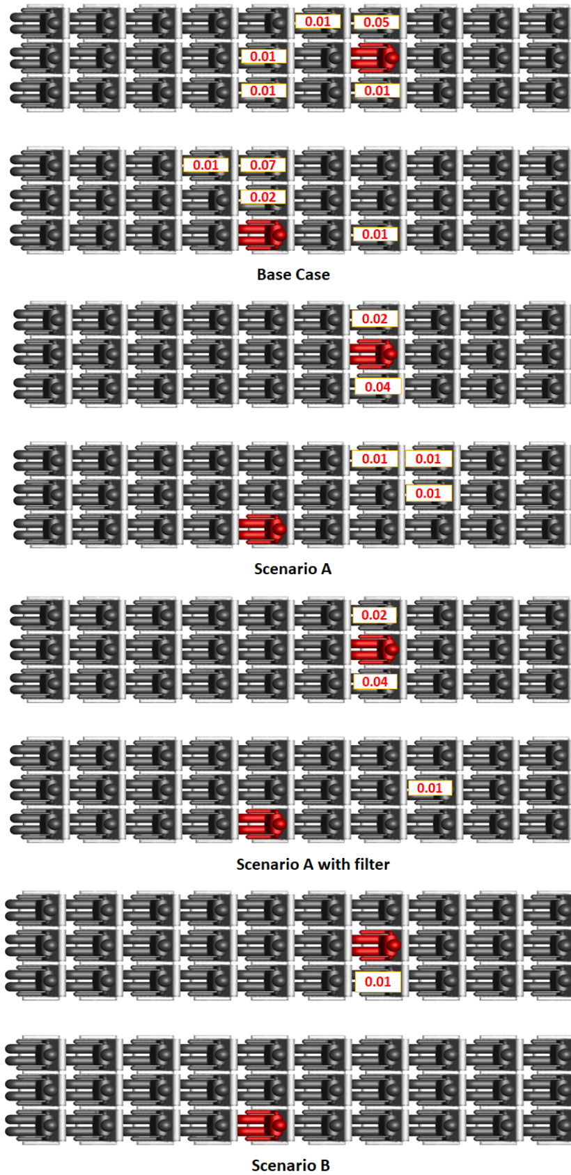
Figure 2. Distribution of potential passengers who are inhaling the aerosol particles released from the infected, red-colored passengers. Red numbers represent the inhaled fractions of the aerosols by susceptible fellow passengers.
